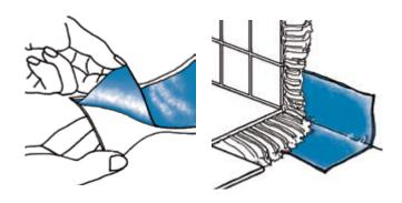
**Domoproof® Elastoband** is compatible with common glues (cement and non-cement based adhesives) and is ideal for use under wood, ceramic coverings. It is highly adhesive, even at low temperatures, to all materials and especially to plastic, glass, steel, polycarbonate and wood. Compatible with most of the bitumen present on the market. The product must be protected from UV rays.
