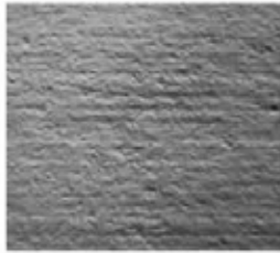
CSP 4 (light scarification)
