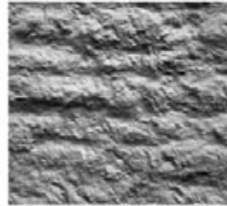
CSP 9 (heavy scarification – rotomilled) abrasive blasting)
